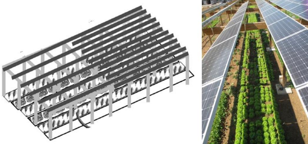
**Figure 27: Montpellier APV System- Left: The sketch of half density and full density settlement. Right: The picture of the field. (Morrou and Guilioni *et al.*, 2013)**
