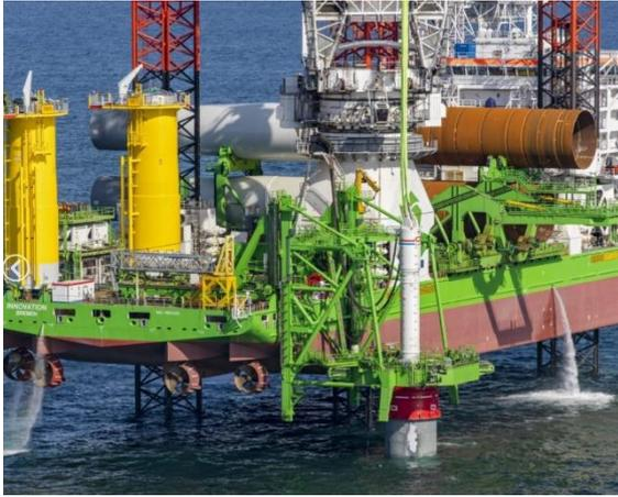
Figure 56 Jack up Barge Vessel with Grippier-Pendulum Attachment
