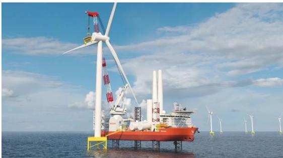
Figure 58 Turbine Installation Example with Jack Up Vessel
