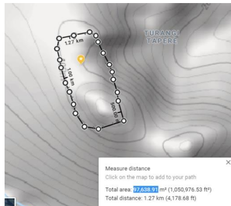
Figure 3.5-8 upper reservoir size calculation using google map
