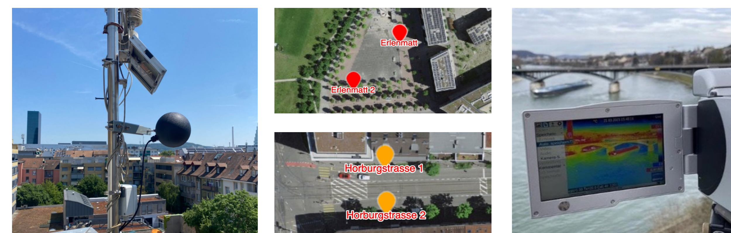
Figure 2: Image of the black globe sensor (left). Example locations of the black globe sensors for the use case "sun vs. shade" (center). Image of the InfraTec VarioCAM HD research 900 used by meteoblue (right).
